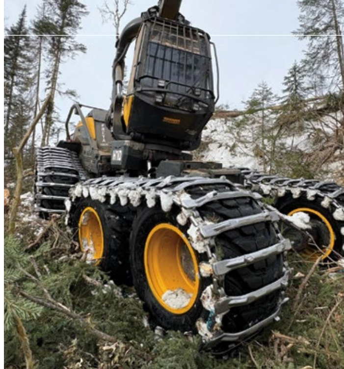
Tracks on the forwarder wheels make for better traction on steep and/or soft ground and decrease soil compaction by driving on processed material. Photo credit: Liam Parfitt, Freya Logging Inc.
