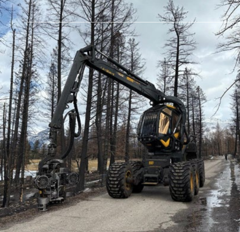
Tracks can be removed from the machine for less soil disturbance in certain conditions or driving long distances.
